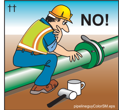
Figure 96 Never straddle or sit on a pressurized pipeline
