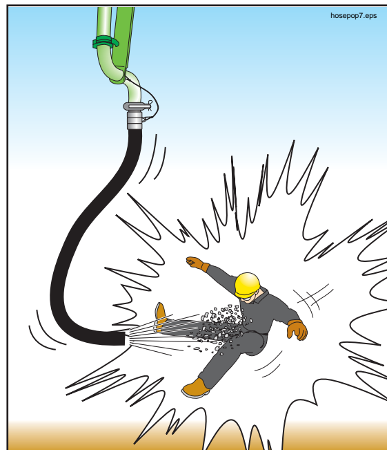
Figure 80 Remove everyone from the discharge area whenever the pump is first starting, restarting after moving, or if air has been introduced into the line
