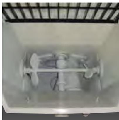
*Fast cleanout with less wasted concrete is a benefit of these SP models over other pumps. The standard hopper agitator keeps concrete flowing to the material cylinders for smooth pumping of even the harshest mixes.*
