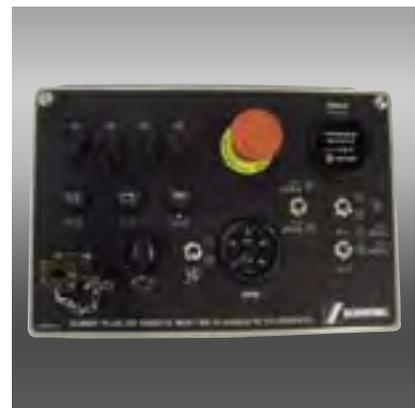
*Convenient control panel includes electric switches for on/off, forward/reverse and agitator on/off. Tachometer and hour meter are also located here along with E-stop, fuse panel and ignition switch.*
